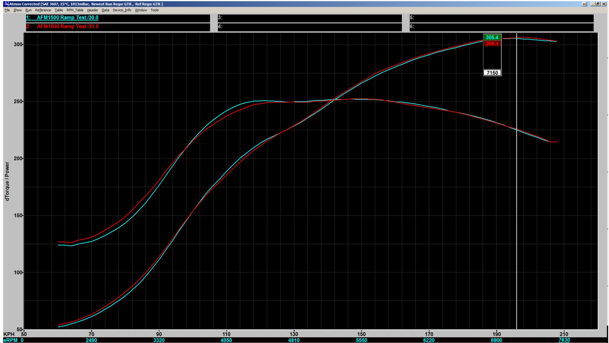
**NOTE:** Power and Torque will “Crossover” at 5252 engine rpm (When imperial units of measure are used)
